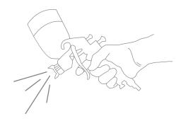
Pressure water cleaning can only be used in the unit's chambers which are equipped with condensate drainage trays. Pressure water cleaning cannot be used for other parts of the air-handling unit. Spray the roof, walls and bottom of the chamber with pressure water and then drain the condensate drainage trays and dry the air-handling unit.
