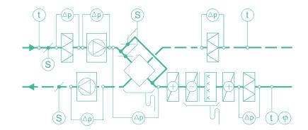
RECOMMENDED COMPOSITION OF AIR-HANDLING UNITS EQUIPPED WITH A HEAT-RECOVERY EXCHANGER
