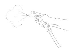
Cleaning is performed using 8-bar compressed air. Compressed air can only be used to remove contaminant from hard-to-access places and to clean components which can be slid out of the unit, such as heat-exchangers. By the effect of compressed air, deposited contaminants are released. During test cleaning, note possible destructive effects on each component of the air-handling unit, such as drop eliminator fins, door sealing, etc.
